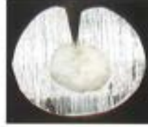
Cross section of solder wire with V-groove.
