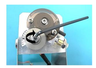
4) Insert the reel axis into the solder wire reel and set it to the reel holder at the bottom.
